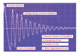
The Decay curve of winding voltage
