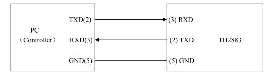
Figure 6-3 Connection of the instrument with PC
