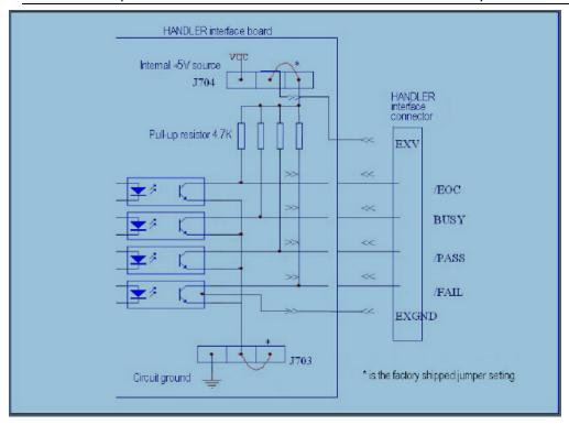
Figure 9-1 Simplified diagram of the output signals
