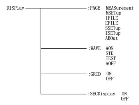
Figure 8-2 DISPlay subsystem command tree
