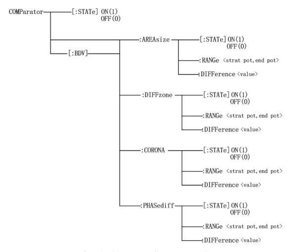
Figure 8-5 COMParator subsystem command tree
