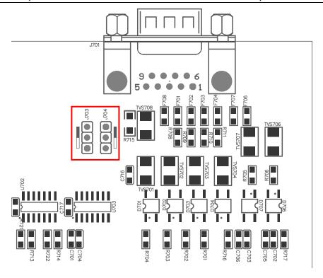
Figure 9-3 Jumper position on the Handler interface board
