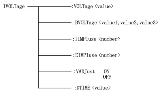
Figure 8-3 Impulse VOLTage subsystem command tree
