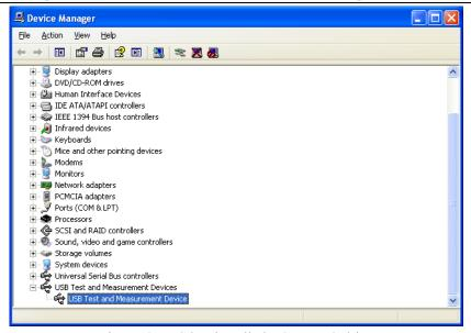
Figure 6-7 PC has installed USBTIMC drive
