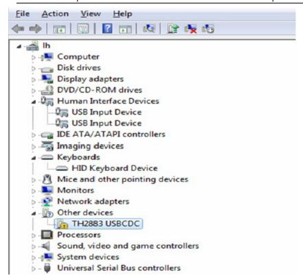
Figure 6-6 USBCDC has not been installed.
