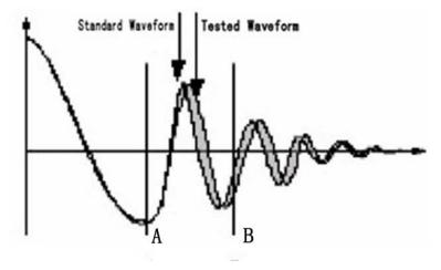
Figure 2-2 Differential Area Comparison
