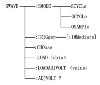
Figure 8-9 Standard WAVE subsystem command tree
