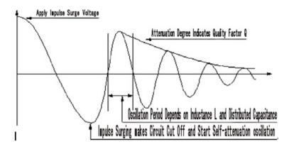
Figure 1-2 Typical self-attenuation oscillation wave
