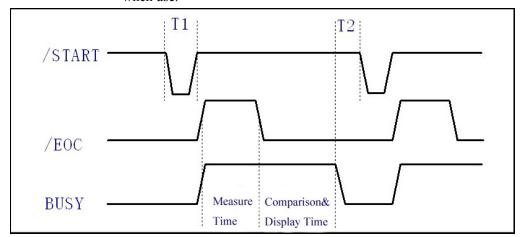
The timing diagram for handler interface is displayed in above figure, T1 is the trigger pulse width and the minimum pulse width is 1 us. T2 is the delay time, after the foregoing measurement completed to next trigger signal; its minimum pulse width is 0 us. /PASS and /FAIL signals are asserted after the measurement completed, till next trigger. The request of the /STOP pulse signal is the same as /START pulse signal.
