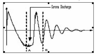
Figure 2-3 Corona Discharge Comparison
