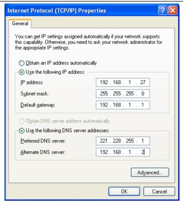
Figure 6-8 Network parameters of Host computer
