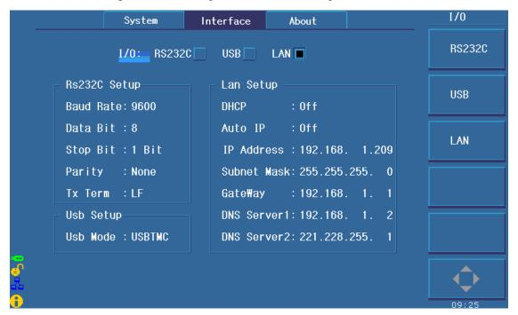
Figure 6-9 Network parameters of TH2883
