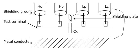
Figure 5-2 Eliminate the influence of stray capacitance
