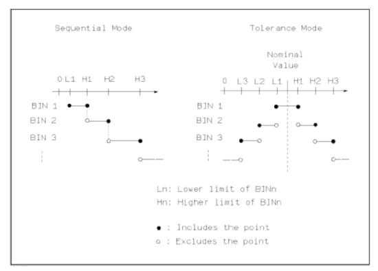
Figure 3-3 Tolerance mode and Sequential mode
