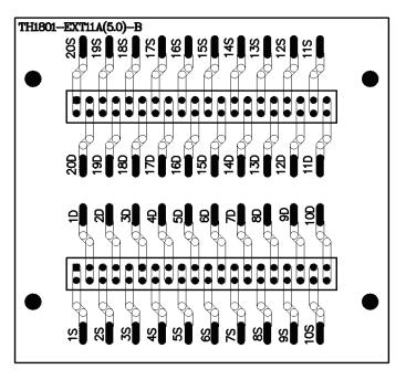
The theory of 4-cable measurement is the test cable of DRIVE and SENSE should be divided. In this figure 1 D means the drive terminal of pin 1, 1 S means sense terminal of pin 1.
