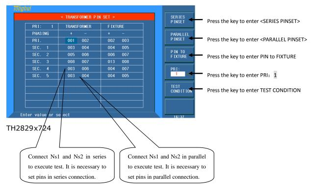
The following figure is the pin setting page of PRI:2 (PRI: 2 is available when Np2 is used as primary winding group.)
