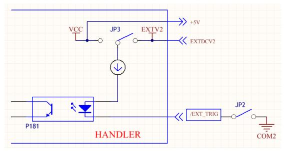
Handler input interface internal diagram
