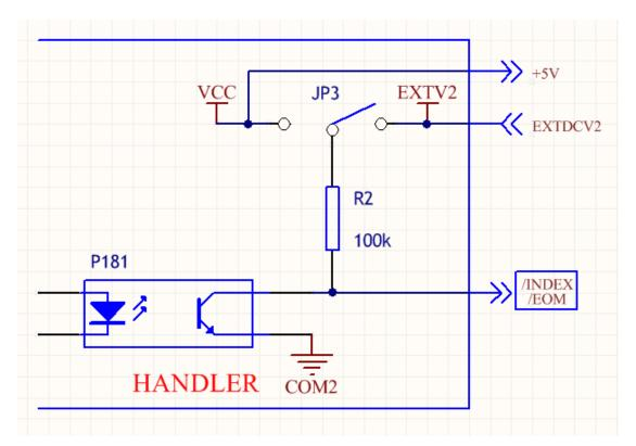
Handler output interface internal diagram 2
