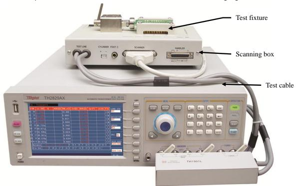
TH2829x702---Connect the scanning test cable to TH2829X
