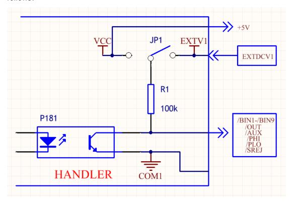
Handler output interface internal diagram 1
