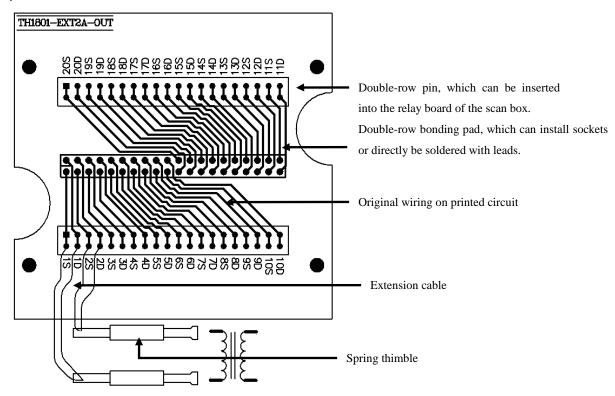
The theory of 4-cable measurement is the test cable of DRIVE and SENSE should be divided. In this figure, 1 D means the drive terminal of pin1, 1 S means sense terminal of pin 1.
